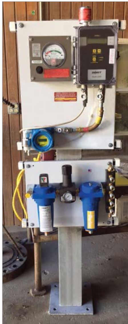
A custom designed AFS-100 air filtration system with a ProAir 2200 carbon monoxide monitor.
