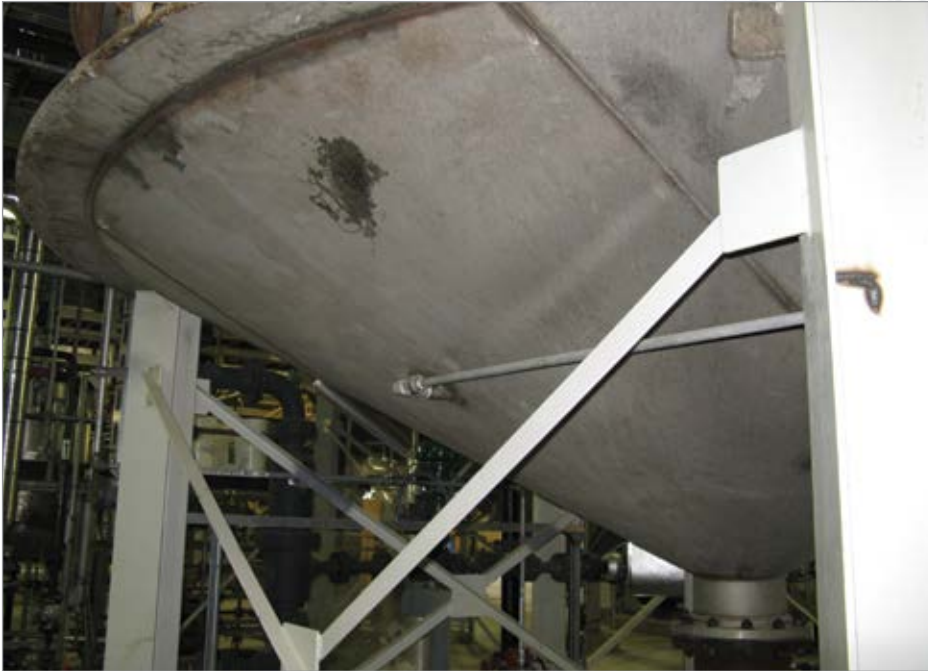
Figure 2: Air is injected into the fermentation process for mixing. This causes a step change in flow.
