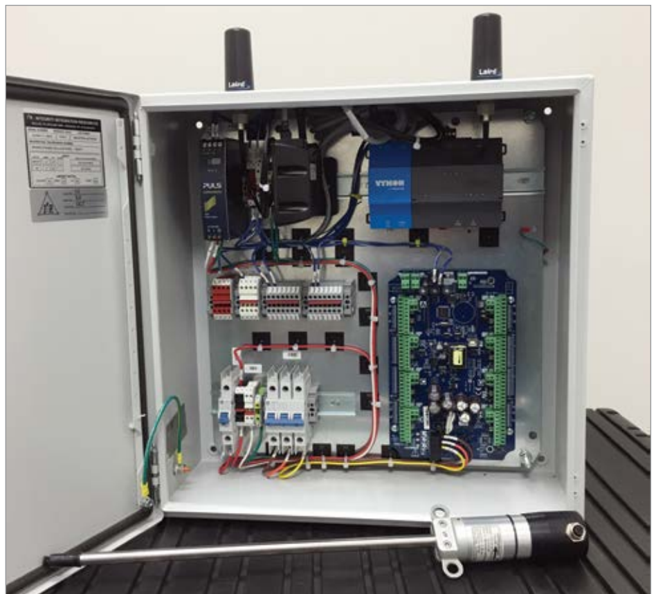
Shown is a typical data acquisition and control panel with a power meter and flow sensor.
