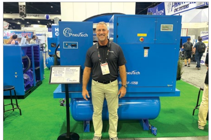
Daniel Schopf of PneuTech with an RK 25F rotary screw air compressor with an integrated refrigerated compressed air dryer.
