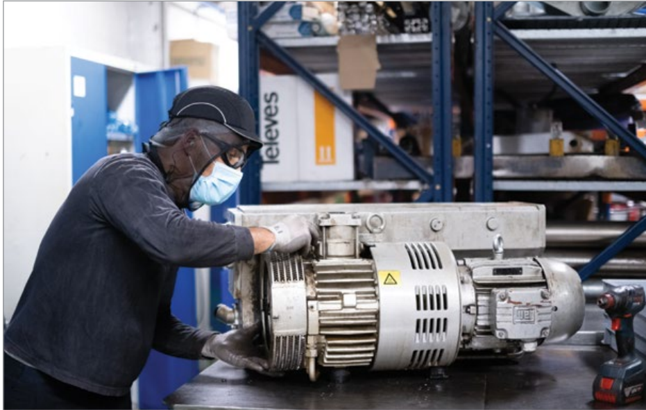
A Klöckner Pentaplast employee gives a vacuum system a high-efficiency motor upgrade.
