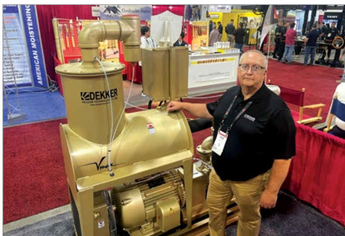
Steve Nash of Dekker Vacuum Technologies with a Vmax 553 liquid ring vacuum pump.
