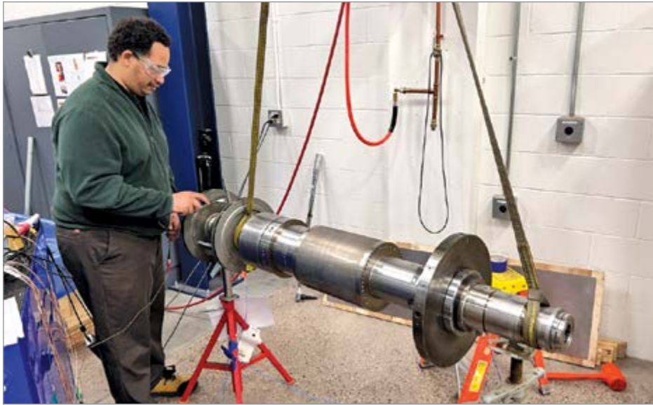
An engineer measures the natural frequency of a shaft by imparting impact with a tuned hammer and measuring rotor response.
