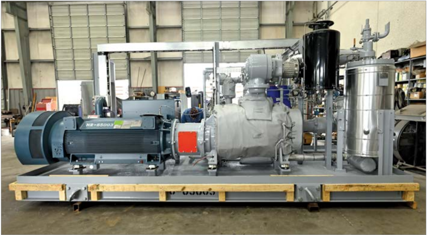
One of three custom-built 550 HP air compressors headed for the north shore of Alaska.
