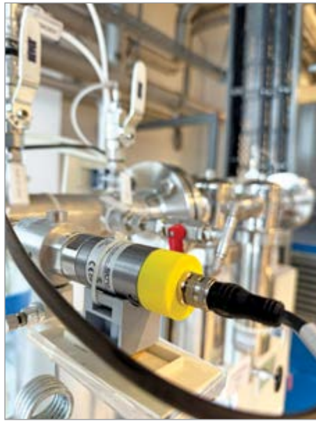
A dew point measurement at system pressure with conversion to ISO 8573 reference conditions.
