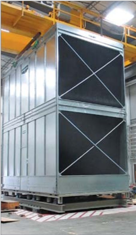
A crossflow cooling tower undergoing seismic shake table testing to validate structural integrity and performance under dynamic conditions.
