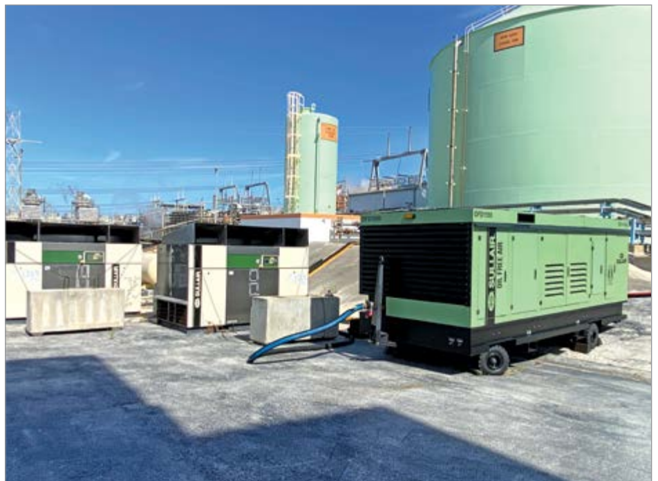
A major utility runs this oil-free portable air compressor and the two older oil-free rotary screw air compressors behind it.
