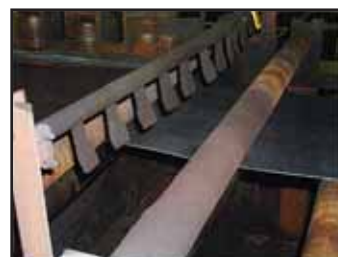
Uncontrolled open blow in a steel plant later replaced with fewer venturi amplifiers
