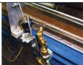
Uncontrolled blow off—later installed photo eye solenoid control for auto shutoff
