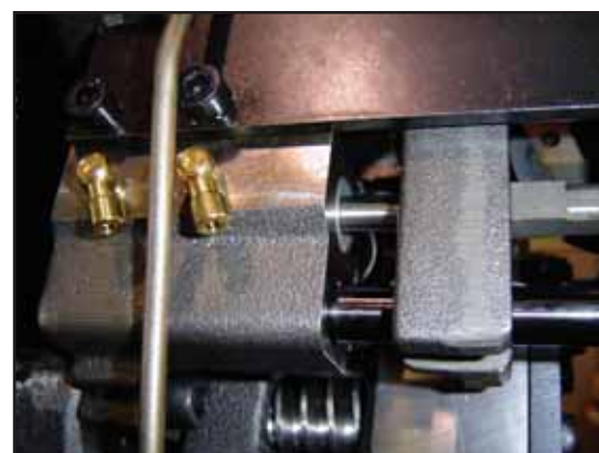
Pneumatic piston controls the position of the blanket cylinder.
