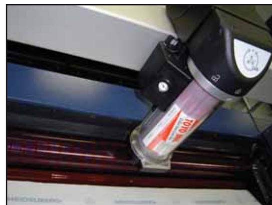
The ink dispensing unit uses pneumatics.
