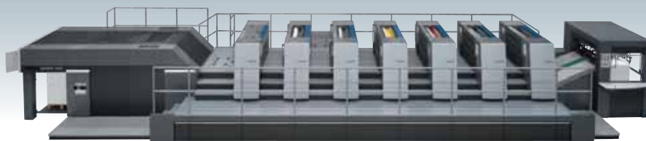
Sheets move from the sheet feeder (far right) through the offset printing units on a Heidelberg XL 105 Speedmaster (Illustration: Heidelberger Druckmaschinen AG).
