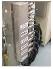
Manifold for Injection Molding — After.
