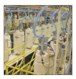
Multiple NovaDrier Compressed Air Resin Dryers Using Membranes from Novatec.
