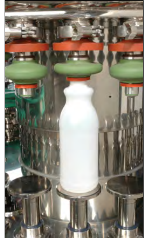
Using pneumatics for washdown applications in the beverage industry is an advantage because of low maintenance costs and reduced downtime.
