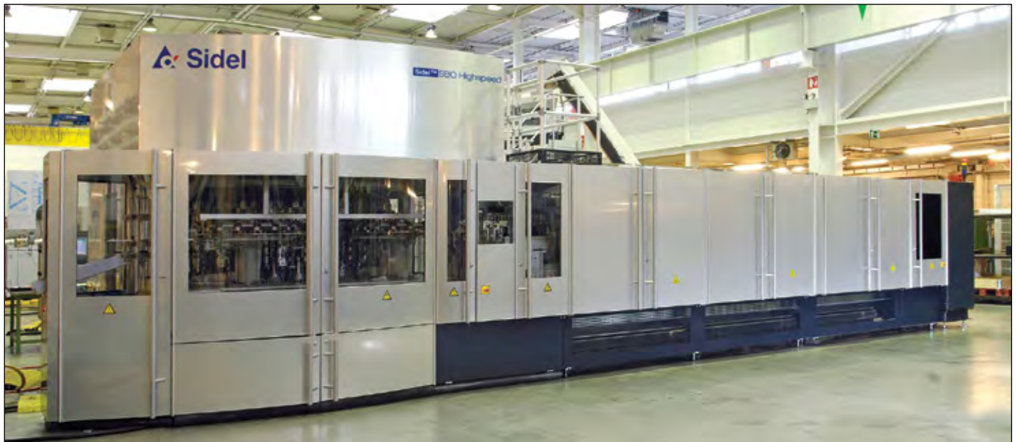
The Sidel SBO 34 Highspeed blows 61,200 small bottles per hour (from 0.2 to 0.7 L).
