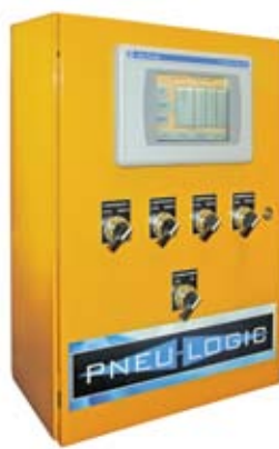
The PL1000 is designed to control up to eight air compressors and to allow management to monitor and trend system performance.
