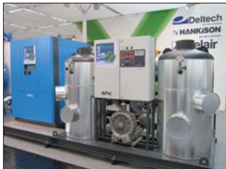
SPX displayed the very energy efficient combination refrigerated and blower purge desiccant compressed air drying system.
