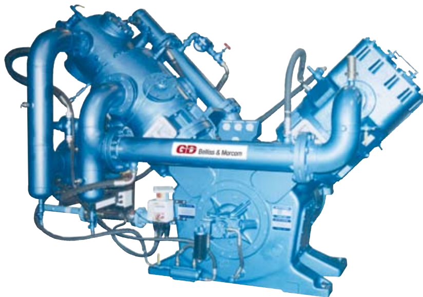
A double-acting piston air compressor compresses air on both the up and down stroke of the piston and is available in multi-stages to provide the higher pressures and air flows required for P.E.T. bottle blowing.
