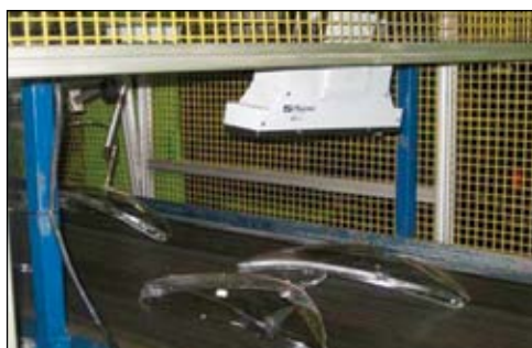
Electric blower replaces compressed air use in headlamp production
