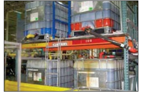
Chemical tanks requiring airlock – reduces compressed air use during lower production periods by installing small dedicated compressor
