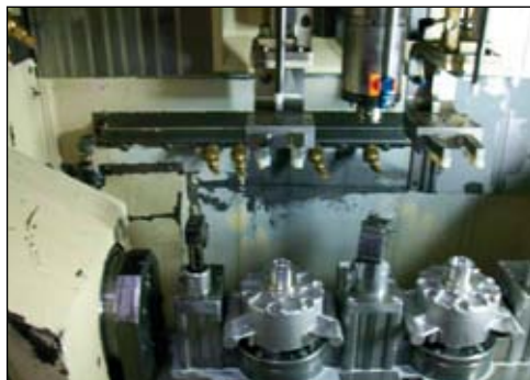
Venturi nozzles installed on open blow-offs reduce compressed air usage
