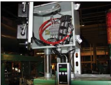
Compressed air flow meters are used on each case erector and flow is displayed and data-logged at a centralized location.
