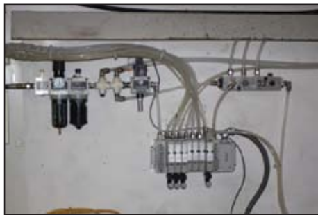
AFTER: Pneumatic circuit on the load center machine consuming the “Best Practice” 23 cfm at idle.
