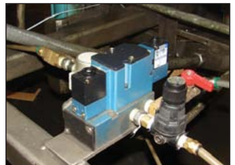
BEFORE: Two 2-position valves consumed 80 cfm when the case packer was idle.
