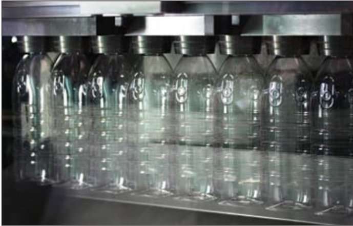
Stretch blow molders operate compressed air systems ranging from 100 psig to 520 psi generating average annual energy costs of $1–$3 million. Image Source: SPI: The Plastics Industry Trade Association
