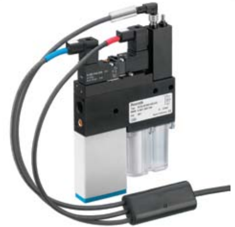
Look for vacuum generators with air-savings options, which have integrated sensors to monitor vacuum levels and greatly reduce air consumption and operating costs.
