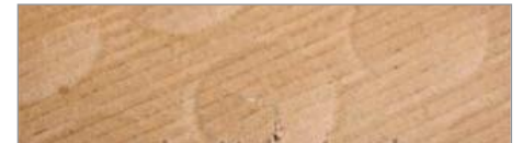
Typical marks/damages from cups on a corrugated cardboard box.
