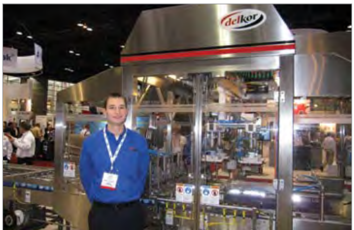
The patented Delkor Spot-Pak® Packaging System uses pneumatics to fire glue guns and compressed air driven vacuum generators.
