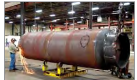
Sparks fly as Shawn Golliher applies welds to a custom air receiver at TIGG's Heber Springs, Ark. manufacturing facility. Thanks to a compressed air audit, TIGG was able to substantially reduce its energy costs.
