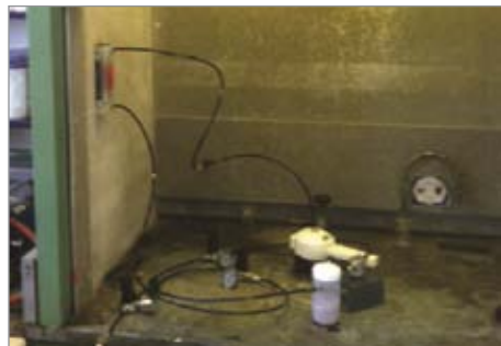
Figure 4: Set up of bacterial nebulization and sampling system
