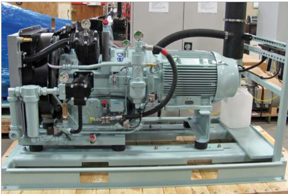
Three-stage, reciprocating piston high pressure air compressor for PET — Sauer Compressors USA, WP271L.
