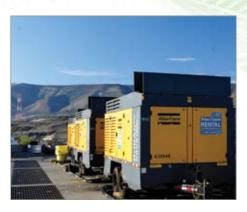
Several Atlas Copco DrillAir TM XRVS 1300 CD7 high-pressure diesel compressors onsite at the Wanapum Dam
