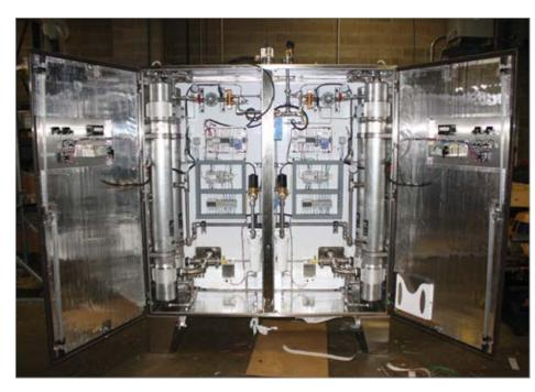
Figure 3: Internal view of the dual nitrogen generation system designed by Titus Air Systems
