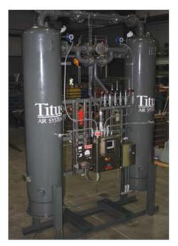
Figure 2: The refinery's Oriad dryer revamped by Titus Air Systems
