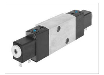
The VSNC is a strong competitor in price, durability, and environmental tolerance. Available as one unit for 3/2 and 5/2 functionality, the switchable seal doesn't require the storage of additional parts to convert the configuration from one operation to the other. Available in 5/3 options, the VSNC can be used for positioning applications and can be ordered with the mid position as closed, pressurized, or exhausted.
