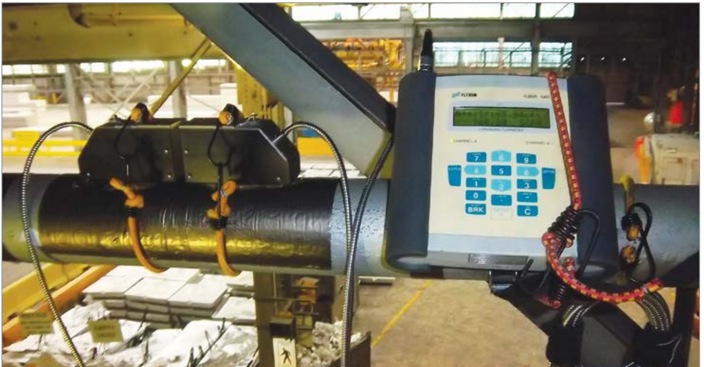
The aluminum plant installed two ultrasonic flow meters — both on the main compressed air headers 60 feet above the floor.
