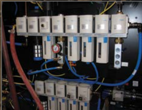
The TRUMPF Trulaser 3030 relies on Festo Compressed Air Regulation and Preparation modules.
