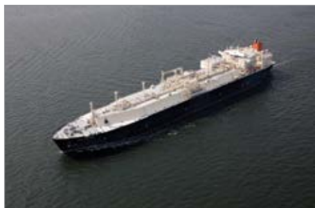
The vessel under construction is a large LNG carrier. The vessel will have a length of 297.9 meters, a breadth of 47.9 meters and a cargo tank capacity of 180,000 cubic meters.
