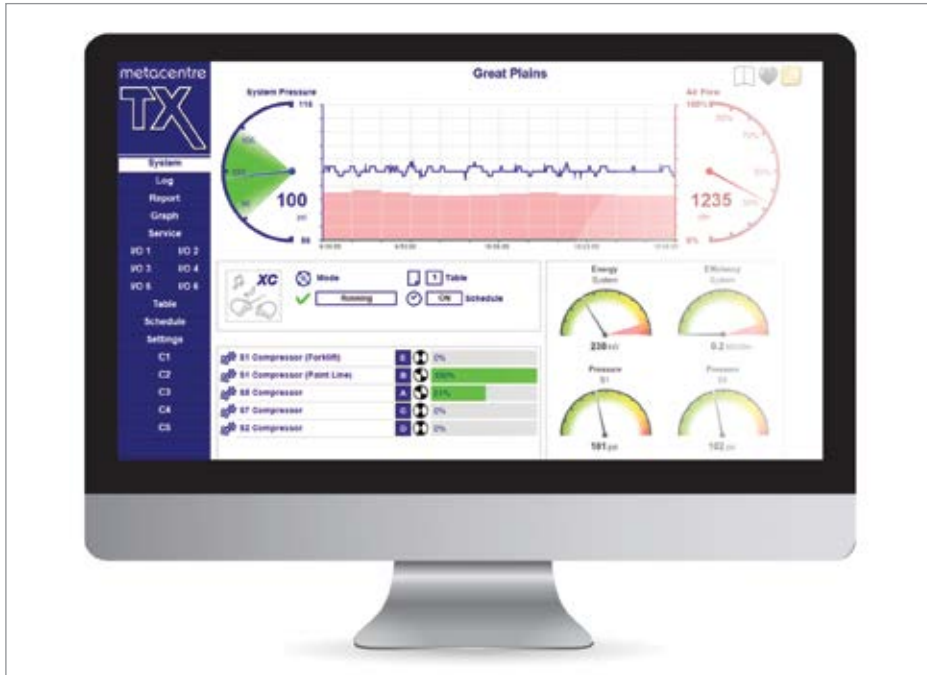
The Metacentre™ XC has the capability to monitor up to two remote pressures from compatible compressor controllers.
