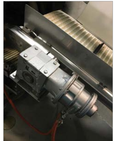
Figure 6: This air motor drives a short conveyor
