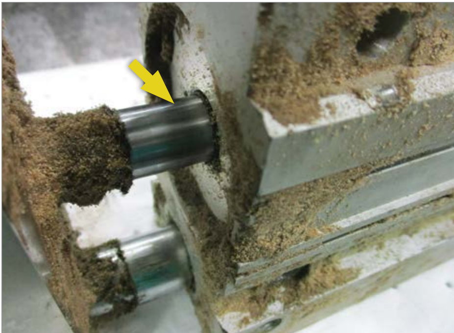
Figure 2: Particulate Ingression Point. (Image courtesy of Motion Industries.)
