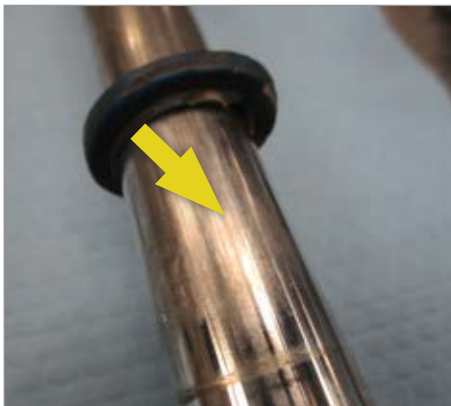
Figure 3: Particles lodged in the rod gland seal and matching scoring on the rod. (Images courtesy of Motion Industries.)
