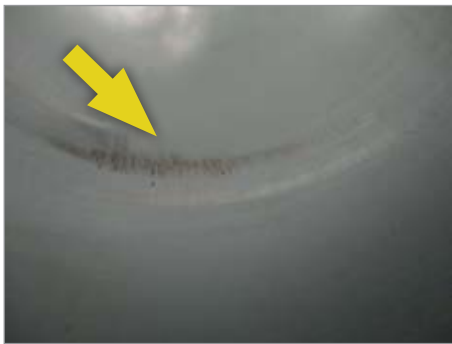
Figure 4: Particles lodged in the piston seals and matching scoring marks in the Barrel. (Images courtesy of Motion Industries.)
