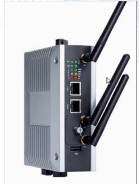
Figure 1: Electronic Monitoring gathers various sensor data and sends it to a cloud database for processing and visualization
