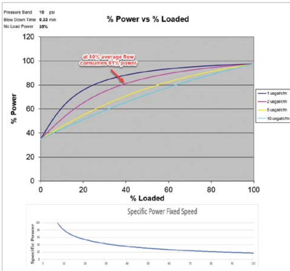
Figure 3: Depicted is power versus flow for load/unload fixed-speed air compressors with various storage receiver sizes. The most common size is about two gallons per cfm of air compressor capacity. The specific power curve at the bottom is for this size storage receiver. Except for the upper range of operation, part-load operation is much less efficient than VFD control.
