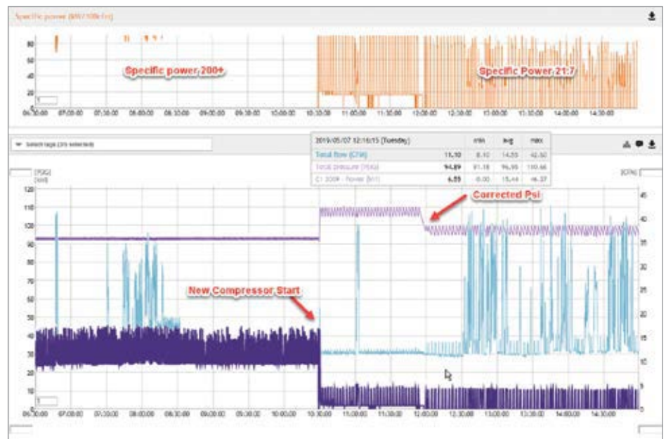
Figure 1: This chart shows pressure (magenta), power (purple) and flow (blue) at a bean processing facility. The power signal is from a common feed, halfway through the sample a new more efficient air compressor is started. Within an hour high pressure and less than optimal operation was detected based on remote readings and adjustments were made to correct the situation before the technician left the site. (Source: CALMS Air.)
