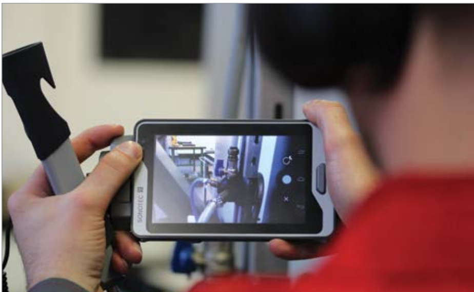
Data collection tools, such as cameras, are often integrated into ultrasonic leak detectors.
