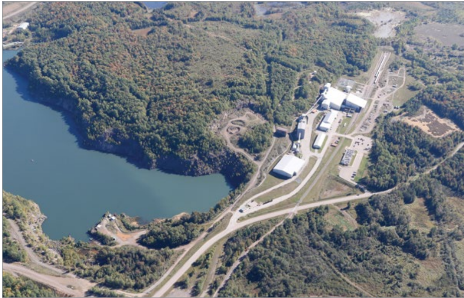
Eagle Mine's processing mill uses crushing, grinding and flotation methods to produce nickel and copper concentrates.
