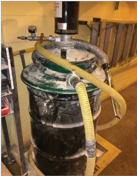
Figure 5. Compressed air vacuums like this can cause high peak demand which trigger an additional compressor to start.
