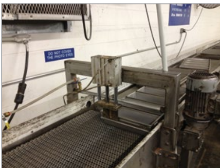
50 Scfm air consumption on homemade air knife used for small bread pans with toppings.
