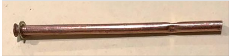
Figure 5: Crimped pipe nozzle from OD 3/16" tube.
