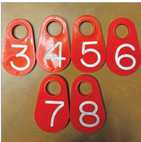
Tags are used to identify compressed air leaks at DENSO’s Maryville facility.
