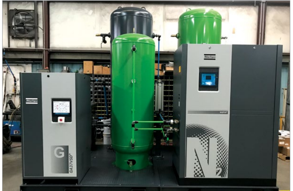
Custom pressure swing adsorption nitrogen generator fabrication project by Arkansas Industrial Machinery
